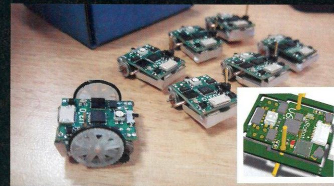
Above Version 6.0 of the micro robot kit is almost ready to go (rendered, above) and includes an accelerator for running the robots on walls: “We have demonstrated the fact that the robots can drive on a ferromagnetic surface mounted to a wall,” Joshua tells us. “The accelerometer will provide all robots with a reliable absolute orientation relative to gravity.”
