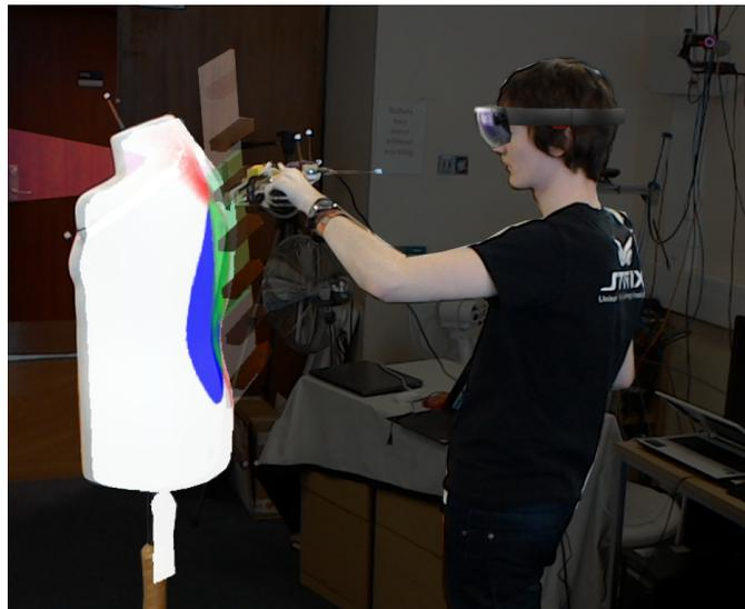
Fig. 1: This figure shows a 3rd person view of a user performing a trajectory using the detailed version of the visualisation. The hand-held robot and the mannequin are motion tracked by an infra-red camera system. This image was taken with the Microsoft HoloLens, and would not normally be visible to a 3rd party. The HoloLens has been added into the image and foreground elements highlighted.
