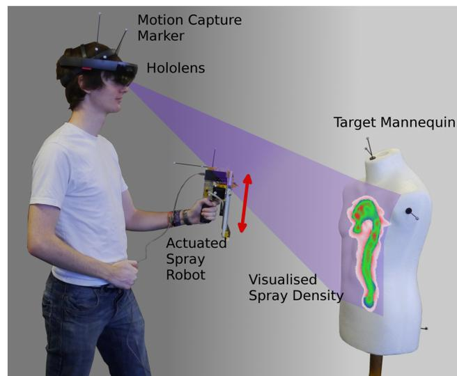
Fig. 1: The experimental setup used in this work. The HoloLens, spraying robot and mannequin all are tracked with retro-reflective markers. The visualisation of the spray density is only visible to the user of the system as it is displayed to them through the HoloLens. The spraying robot’s head can be actuated up and down to assist with the spraying task.
