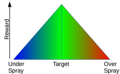
Fig. 4: The colour scheme for a region that requires spraying. Blue would indicate to the user that they should spray the area more, green that the area is correctly sprayed and red that it has become over sprayed. The vertical height in the image refers to the reward that is applied to the whole spraying job at this location, when the score becomes negative the colour will stay red.
