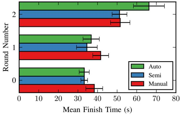
Fig. 6: The time to complete the spraying task. Time is taken from the interval between 10% and 90% of the maximum score for that run to remove unproductive time at the beginning and end of each run. The error bars represent the standard error of the mean (SEM). There is little difference in completion time with different assistance levels.
