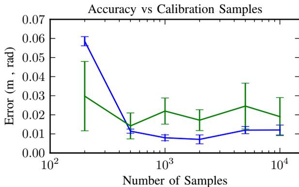
Fig. 3: The error between the measured location of a motion tracked marker and intended position against length of calibration series. Error bars represent the standard deviation in the measurement.  $N=10$  for each experiment. After 500 samples there is no discernible improvement.
