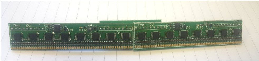
Figure A.1: The custom LED array used for debugging the XAAR 128 interface.
