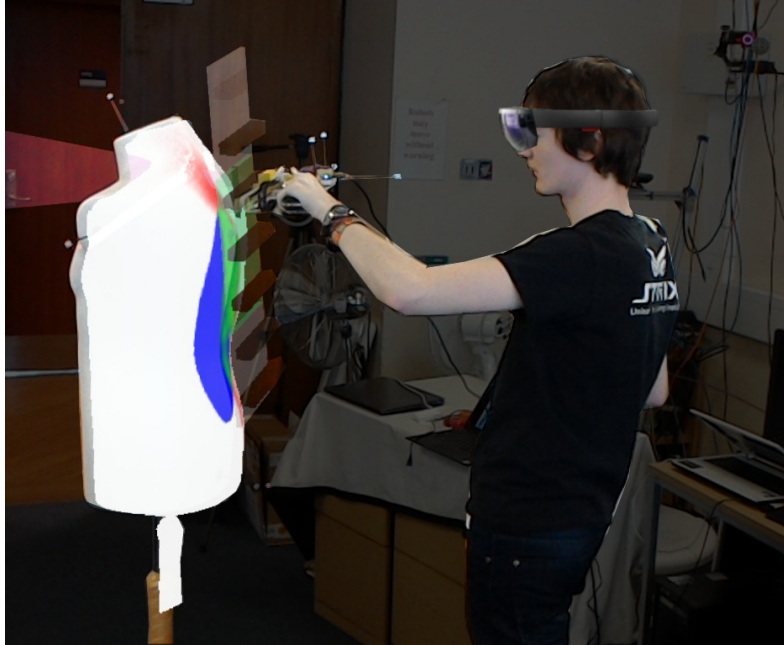
Figure 5.1: This figure shows a 3rd person view of a user performing a trajectory using the detailed version of the visualisation. The hand-held robot and the mannequin are motion tracked by an infra-red camera system. This image was taken with the Microsoft HoloLens, and would not normally be visible to a 3rd party. The HoloLens has been superimposed over the image and foreground elements are highlighted.
